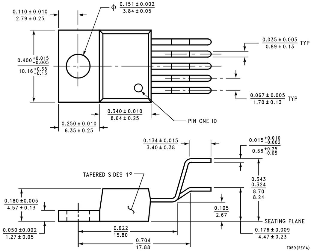
**TO220 5-lead, Molded, Stagger Bend Package (TO220-5)
