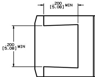
**TO263 5-Lead, Molded, Surface Mount Package (TO263-5)**
