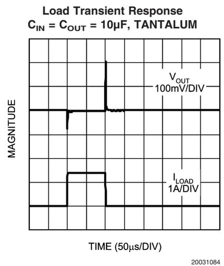
**Typical Performance Characteristics** Unless otherwise specified:  $T_J = 25^\circ\text{C}$ ,  $C_{OUT} = 10\mu\text{F}$ ,  $C_{IN} = 10\mu\text{F}$ , S/D pin is tied to  $V_{IN}$ ,  $V_{OUT} = 2.5\text{V}$ ,  $V_{IN} = V_{O(NOM)} + 1\text{V}$ ,  $I_L = 10\text{mA}$ . (Continued)
